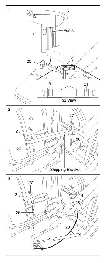
4. See the inset drawing. Remove the rubber bands from the screws. Be sure that the Arm Brackets (31) inside the tubes on the left side of the Base (1) are pressed against the indicated sides of the tubes.
